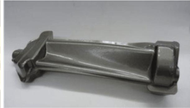
Fig. 9 Forged LPT blade stage 3 for PW1134G
