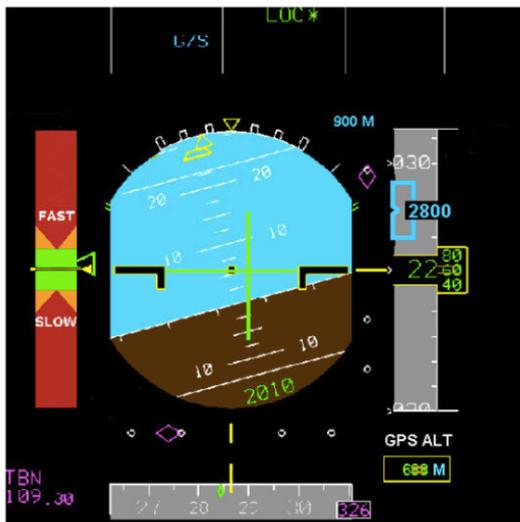
**Airbus Back-Up Speed Scale (BUSS) option replaces the normal PFD speed- and altitude tapes with AOA and GPS ALT when all ADRs are switched OFF.**
