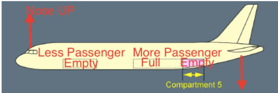
Airbus is working on reprogramming the software which controls the elevators to keep the aircraft flying in a safe flight envelope. Till then the directive is a temporary fix to mitigate the risk.
